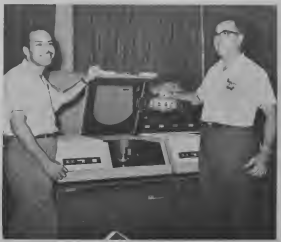
RENE WOLF and Henfilh Fradi demonstrate how disk pack containing operating system is mounted on disk storage drive. The use of disks for direct access to information is one of the outstanding features in the new 360 system.
